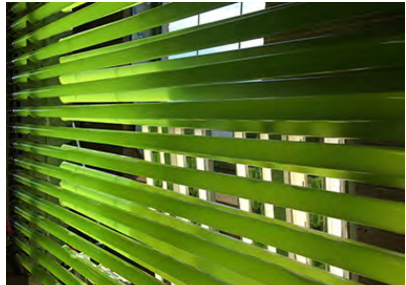
Glass photobioreactors grow algae in circulating water with light, nutrients, and CO 2 captured from Whiner's brewing process.
